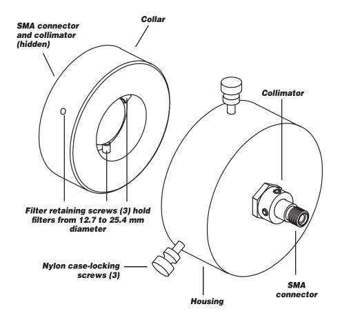
WPI's In-Line Fiber Optic Filter Holder allows insertion of optical filters within a fiber optic pathway. The connectors of the filter holder assembly are compatible with WPI's range of fiber optic jumper cables and can be coupled using SMA (WPI **#56200**) and ST (WPI **#56300**) connectors.
